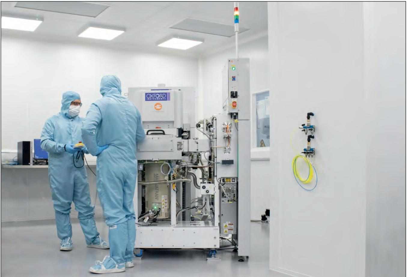
For many years, Plasma Technology has offered tools for inductively coupled etching. Very recently, they have been complemented with equipment that can remove material by one atomic layer at a time. Together, these two etching techniques are ideal for the production of normally off AlGa<sub>N</sub> HEMTs, which have very thin layers, and a two-dimensional electron gas that must not be damaged
